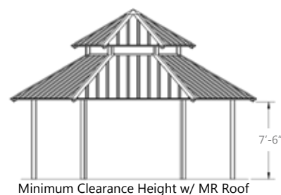
Minimum Clearance Height w/ MR Roof
