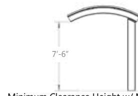
Minimum Clearance Height w/ MG Roof
