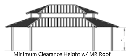
Minimum Clearance Height w/ MR Roof
